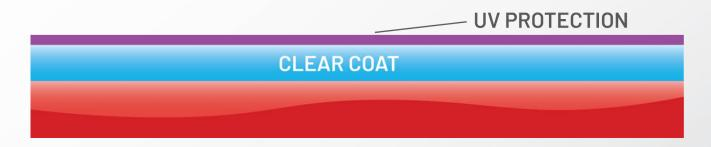
That's right — nearly all of the paintwork's UV protection is in the top layer of the clear coat. Remove that protection, and your clear coat becomes far more susceptible to UV oxidation, which obscures the paint's gloss.
